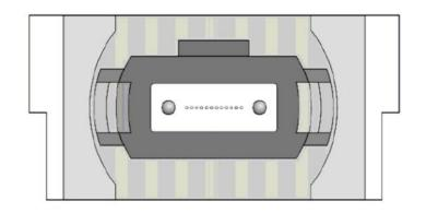
Transmit Channels: 1 2 3 4 Unused positions: x x x x Receive Channels: 4 3 2 1
